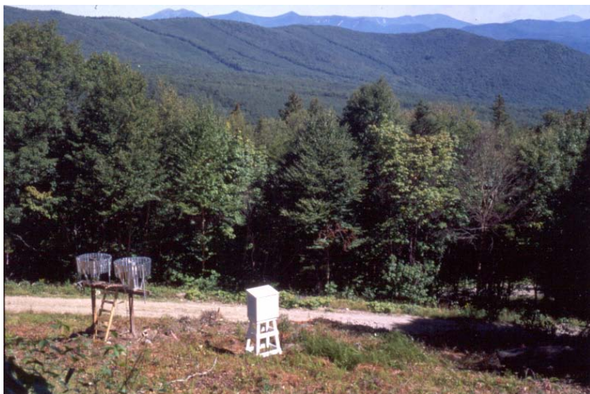
Precipitation collectors to measure water inputs
