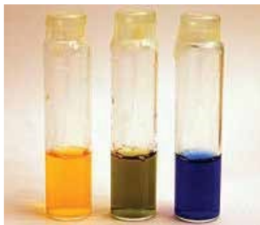
Bromothymol Blue indicator in acidic (yellow = pH 6.0), neutral (green = pH 7.0), and basic (blue = pH 7.6) conditions. Photo credit: http://en.wikipedia.org/wiki/Bromothymol_blue
