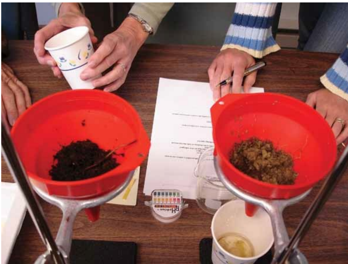
Comparing the flow of water through different soil types
