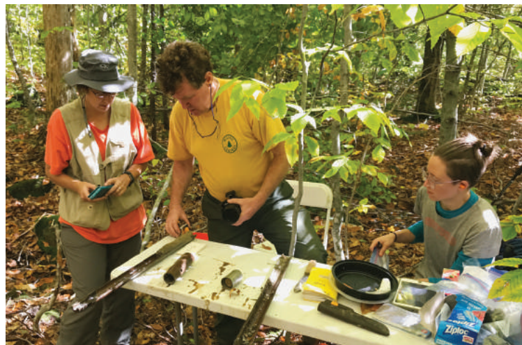
At the top of Watershed 3, Scott Bailey (center), Maddy Schreiber (left), and Jenny Bower, University of Vermont Ph.D. student (right), process a sample core of glacial sediment that is more than 23 feet deep.
